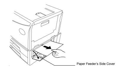
Figure 5.1 Paper jam in paper feeder unit
